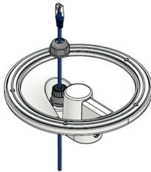
2. Pass the cable through the cable gland
