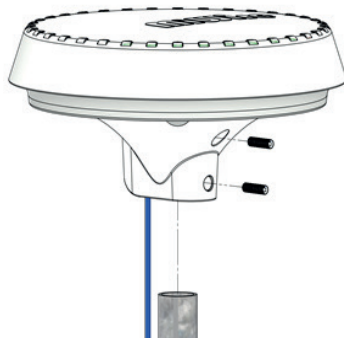
5. Tighten the mounting bracket to a Ø38mm pole
