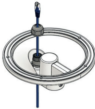
2. Pass the cable through the cable gland
